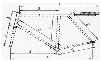
Masse: A =150 - 180 mm B =395 - 455 mm C =560 - 610 mm D =500 - 550 mm E = 400 - 500 mm F =370 - 410 mm G =360 - 410 mm H =815 - 960 mm J = 530 - 580 mm K = 920 - 970 mm
